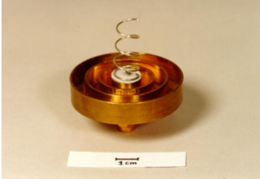
Figure 2.11: Photograph of a 9 GHz model with a triple slotted “soft” groundplane. Note that this photo shows a shorter helix than that corresponding to the measurements discussed here. The measured model had a seven turn tapered helix.
