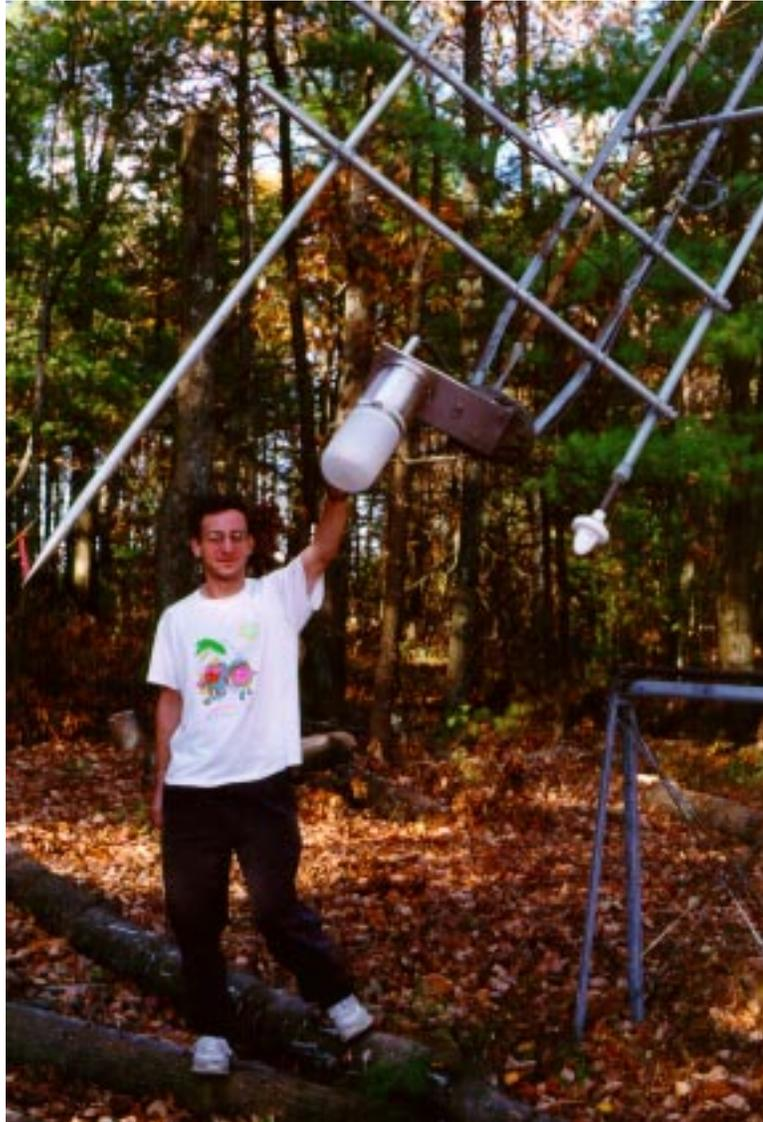
Figure H.8: The GPS antenna, lightning rod, discone and terrestrial feed system mounted on the tower. The tower is tilted down for maintenance.
