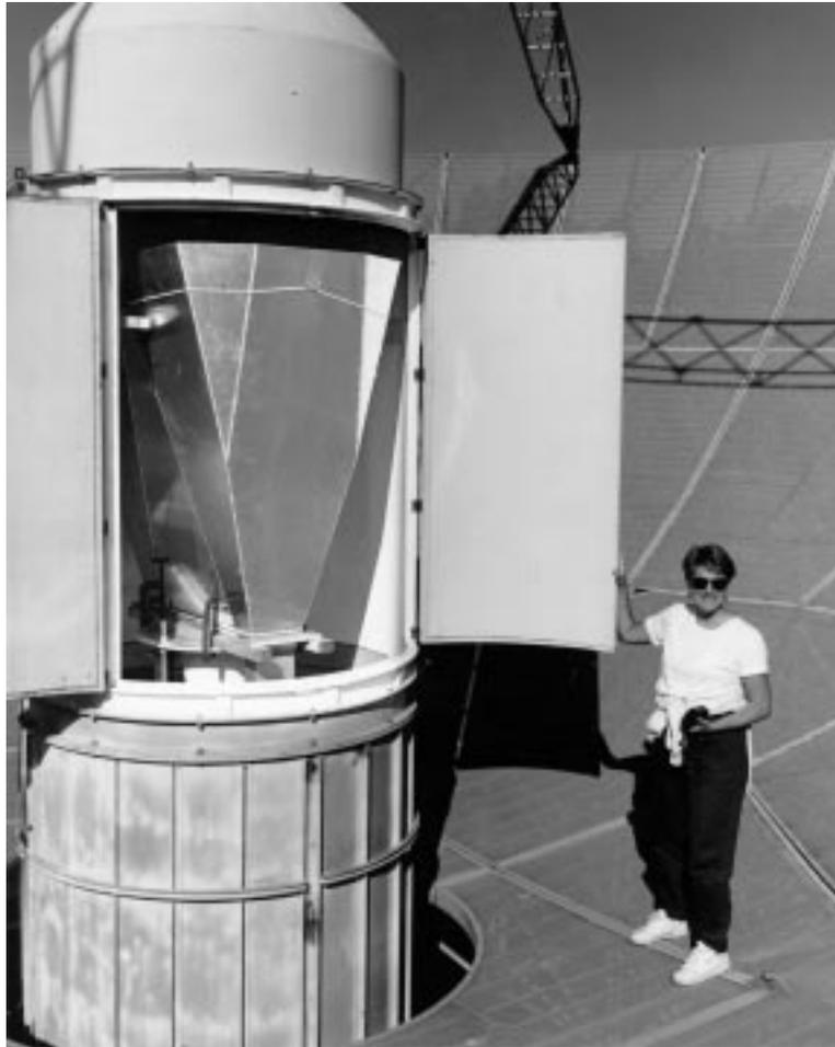
Figure H.6: The sky horns installed in the radome.
