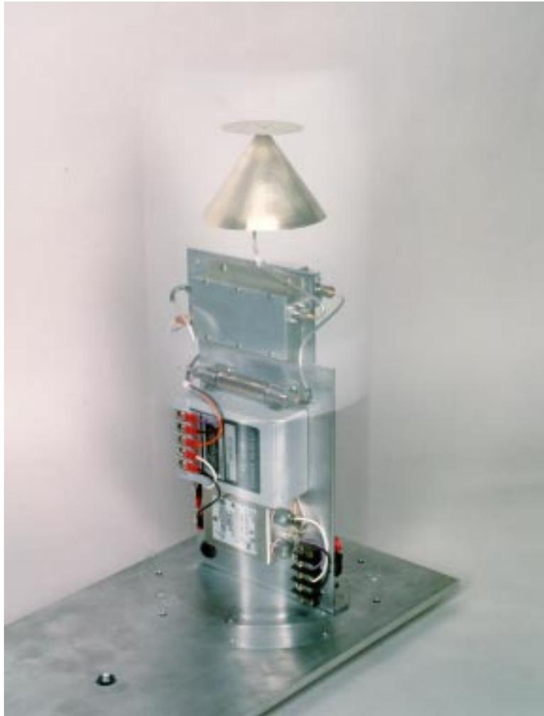
Figure H.7: A double exposure showing the terrestrial discone and its downconversion circuitry as well as its enclosure.
