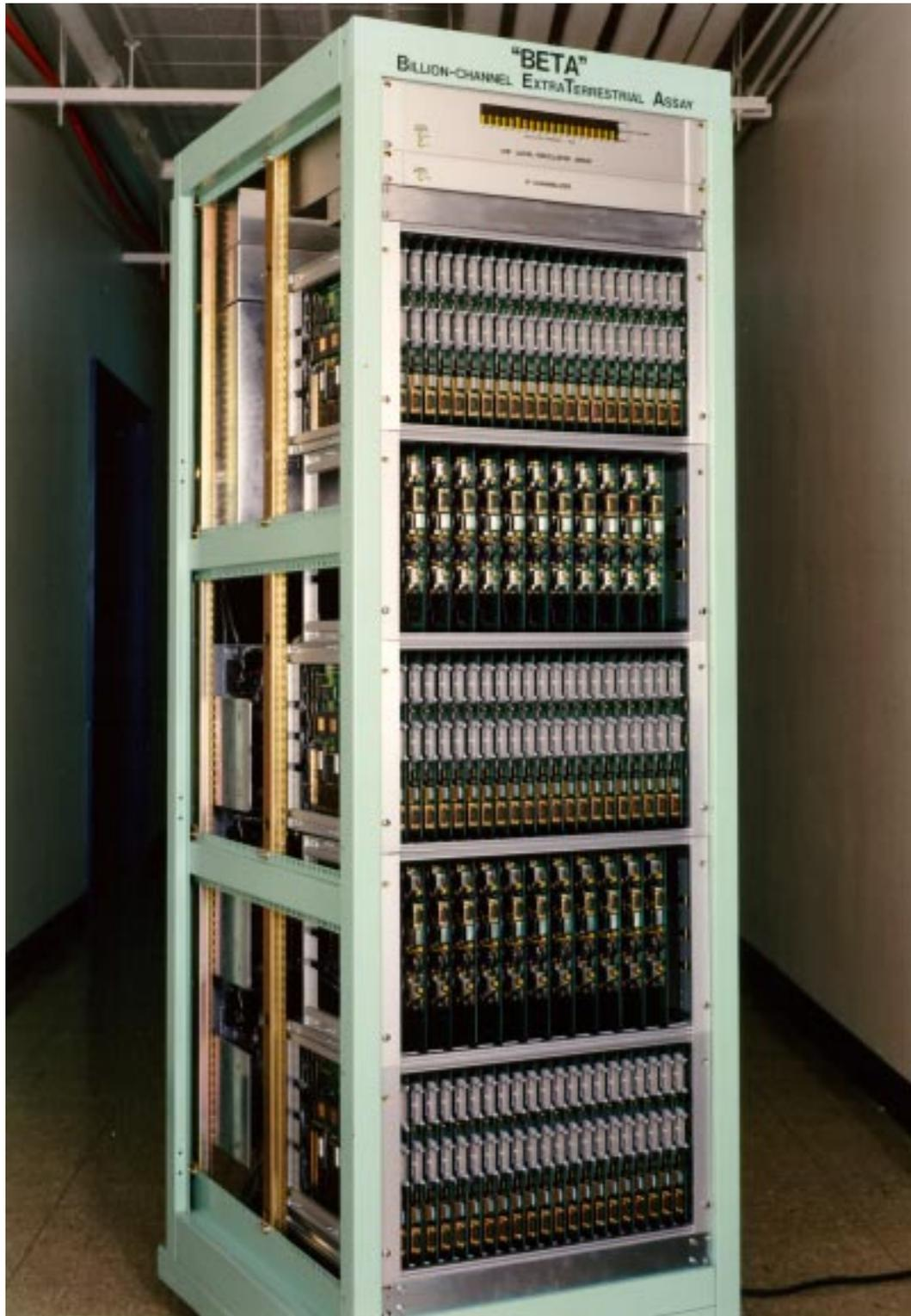
Figure H.16: The *BETA* supercomputer in its rack. The rack holds 63 4M-point FFT boards, 21 mixer-digitizer boards, power supplies and cooling fans.
