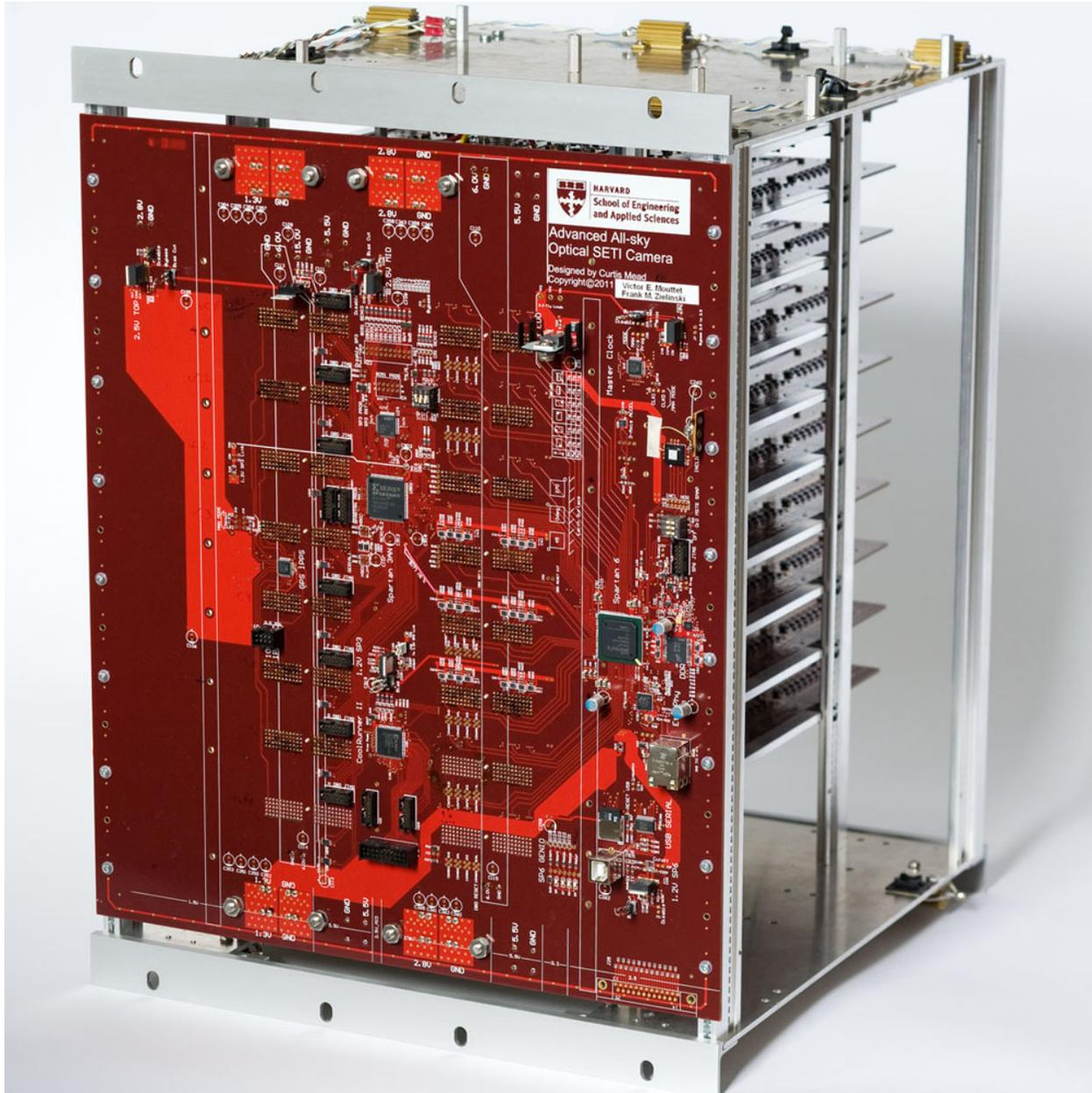
Figure 4.11: The motherboard distributes power and global signals to the daughterboards. A Spartan-6 on the board functions as the system-wide trigger for the 32 PulseNets-V's. Photo Credit: Paul Horowitz.
