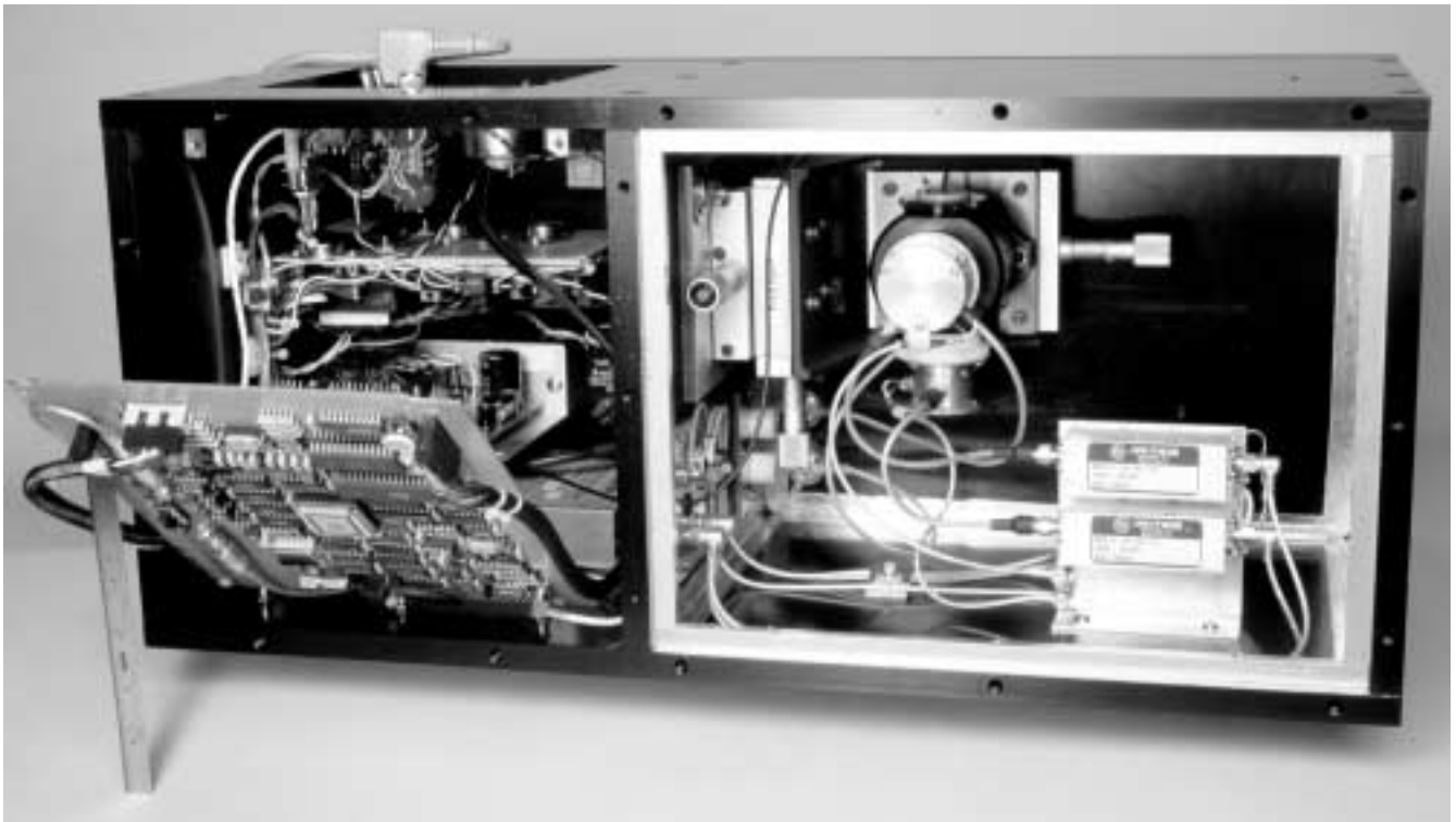
FIG. 2.— The Harvard targeted search photometer, with covers removed. Light enters from the rear of the righthand compartment, focused onto a 30 arcsec aperture, then passes through a beamsplitter onto the pair of HAPDs on their 3-axis stage. The detectors run at a gain of \sim 4 \times 10^4 , producing \sim 50 \mu\text{V} negative pulses into 50 \Omega , which are amplified and sent to the electronics in the lefthand compartment. The latter perform coincidence, 4-level ADC, timing, logging, hot-event veto, and communication with the host Linux PC. The photometer measures 25 \times 25 \times 60 cm, and weighs 30 kg.
